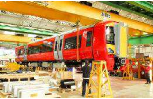
A completed carriage being lifted through the workshop and placed on two sets of wheels.
